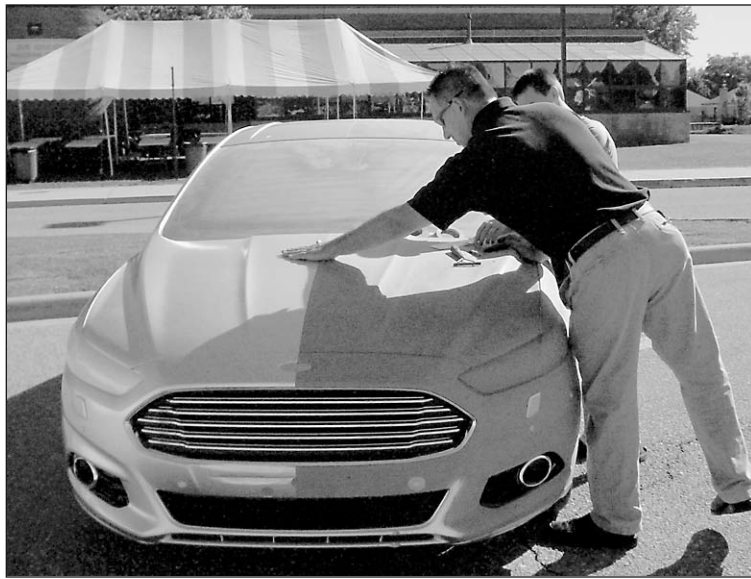
Ford Master Modeler Tom Drobek demonstrates sculpting on the clay model that evolved into the 2013 Ford Fusion.
