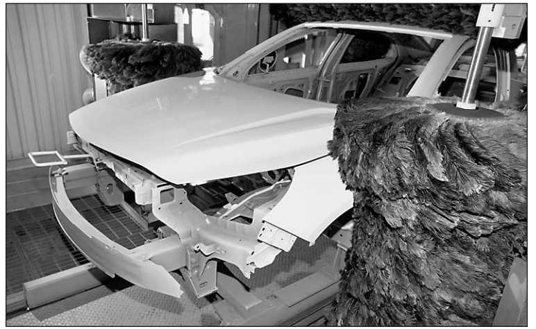
A not-yet-assembled Chevrolet Volt makes its way through a bank of female ostrich feathers at Detroit-Hamtramck Assembly.
