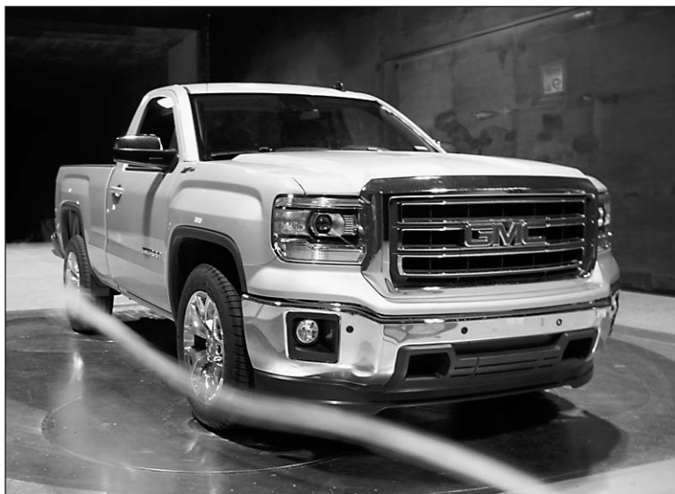
The 2014 Sierra undergoing wind tunnel tests.
