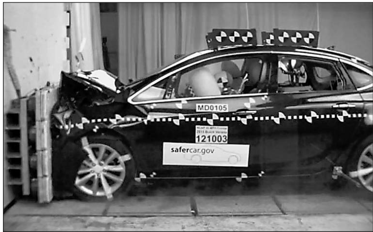
The 2013 Buick Verano is shown in a NHTSA frontal collision test, one of three tests required to gain a 5-star Overall Vehicle Score rating.
