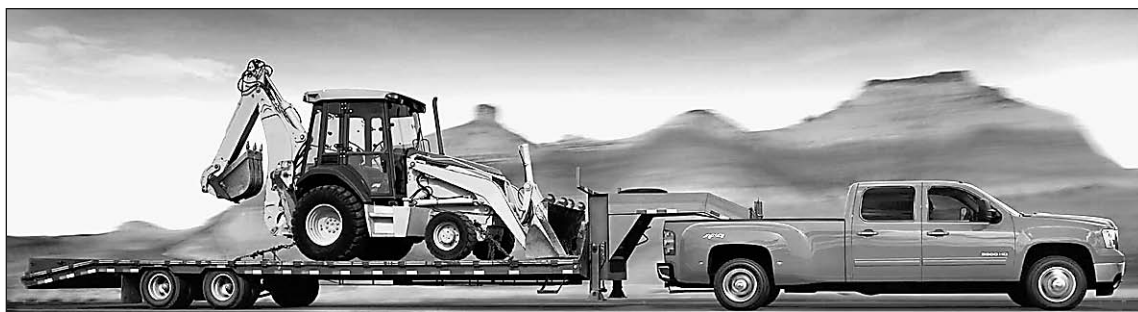
A pickup pulling a flatbed and a John Deere 410e. Note the axle positions and the weight on the gooseneck.
