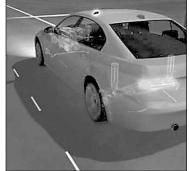
Lane keeping assist tracks lane markings and puts torque on the steering wheel to guide the car back to the center if it strays.
