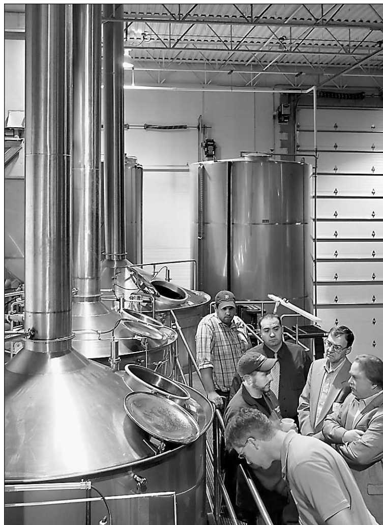
The Auto.Tech.Connect group met Thursday at the Rochester Mills Production Brewery. Marketing Director David Youngman, center with cap, explains the process in the brewhouse area, where the brew kettle, mash tun, lauter tun and hot-and-cold "liquor tank" are located.
