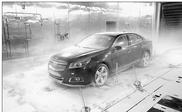
The 2013 Chevrolet Malibu Turbo in the GM Climatic Wind Tunnel.
