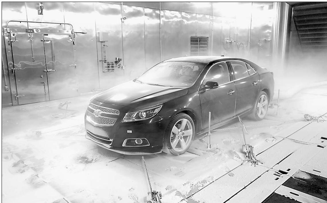
The 2013 Chevrolet Malibu Turbo endures sub-zero conditions in the GM Climatic Wind Tunnel.
