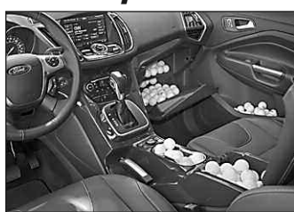
Engineers use pingpong balls to measure cargo dimensions.
