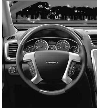
Acadia’s Head’s Up Display (HUD) works by projecting information from within the dashboard, using two mirrors to reflect a crisp digital image off the windshield so that it appears to the driver to be floating in front of the vehicle’s bumper. It was developed from aerospace technology, available on the Acadia midsize crossover, standard on Denali.
